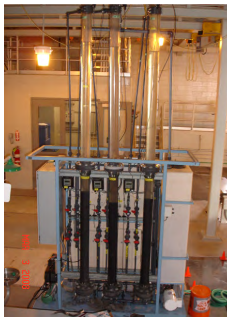
Pilot-scale carbon filters for EDC/PPCP removal.
