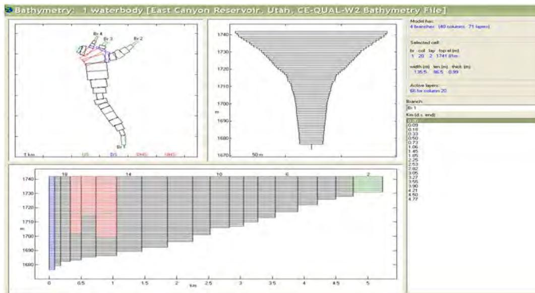
**Figure 1.3.1-1 AGPM diagram of the East Canyon bathymetry configuration. The reservoir canyon walls are very steep in the lower half of the reservoir to near vertical near the dam (top right panel). The shallow littoral areas are primarily found in the inflow segments (2-6- bottom panel) closest to East Canyon Creek, or in the back of branches.**
