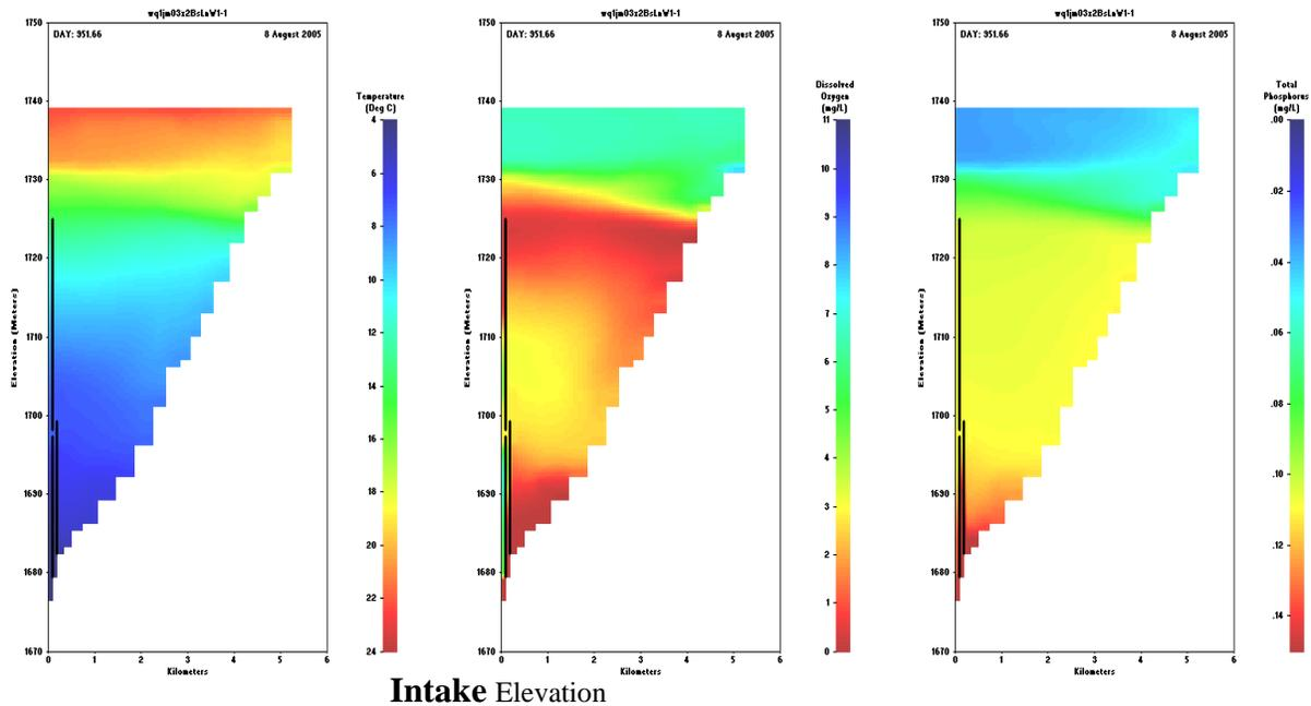
**Figure 1.3.4-2 is an AGPM animation cross section snapshot of three frames depicting temperature, dissolved oxygen, and total phosphorus concentrations. It also illustrates the configuration of weirs and curtains in W2 used to simulate two intake elevations mixing to the single dam outlet at elevation 1687 (M). Phosphorus accumulates for several years in the stagnant hypolimnion zone until it spills through the hole in the old concrete dam (frame on right). The left wall is the dam.**
